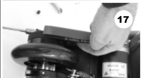
17. Retighten both axle adjusters the same number of turns as noted in #4. This should retension the drive belt and approximately maintain the proper centering of the wheel.
