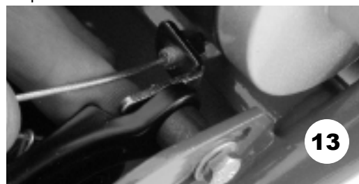
12 & 13. To hook up the brake anchor arm and cable. Align the cable guide adjuster and install the spacer and bolt. Do not tighten until after step 19.
