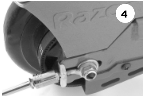
4. Loosen the axle adjusters on both sides an equal amount, about five turns.
