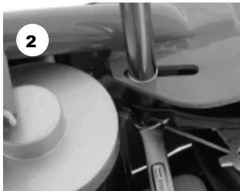
2. Loosen brake arm anchor and remove
