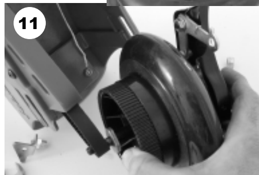
11. Install new wheel. Maneuver the belt onto the wheel pulley and slip the axle into the slots on the frame.
