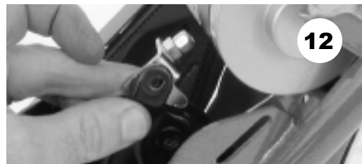
12 & 13. To hook up the brake anchor arm and cable. Align the cable guide adjuster and install the spacer and bolt. Do not tighten until after step 19.
