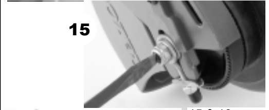
15 & 16. Install the axle adjusters and axle nuts. Tighten until they just hold the hardware in place.
