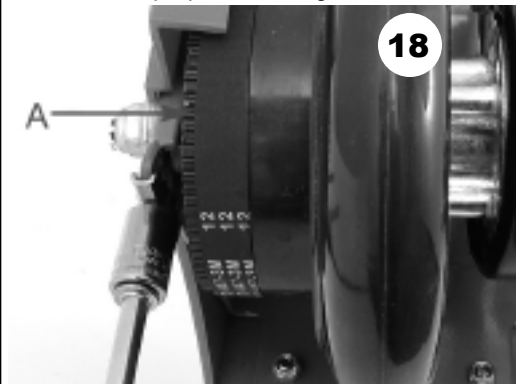
18. Rotate the wheel several times (clockwise when looking at the pulley side). The belt may drift or "track" to one side of the pulley or the other. In example #18 it is tracking to the inside. You want the belt to track to the center as shown in #19. Turn the belt-side adjuster 1/16 to 1/8 turn to track the belt to the center. Watch the belt tension. If too tight, loosen the other adjuster to equalize the wheel and belt alignment.
