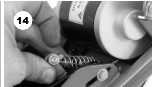
14. Insert the brake spring and thread the cable wire into the cable anchor. Thread the cable to its original position and tighten securely.
