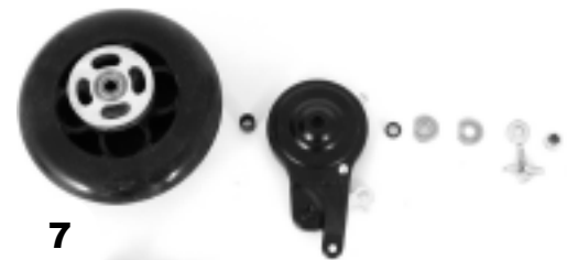
6. Pull the old wheel out. Note the arrangement of the hardware sequence below (7 ~ 10)
